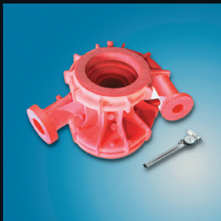
Wax-infiltrated sintering for investment casting (Ø270[+ flange]x295)
